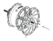
3. Mount the stop pin into on the shaft.
