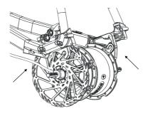
5. Mount the 2mm washer on both sides of the frame.
