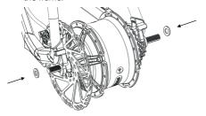
Tighten the flange nuts with open spanner at both sides of the motor. (torque requirement: 47-60 N.m.)
